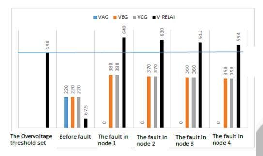
\*) Determined at VT ratio 220/48, based on voltage measurement on the disturbance point
