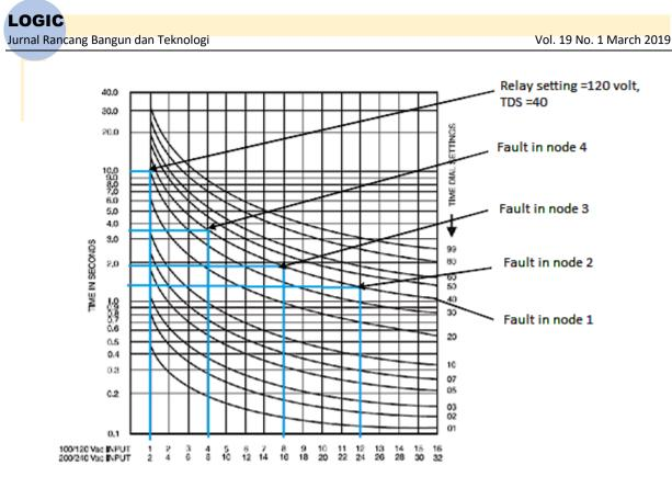
Figure 7 The Characteristic of The Overvoltage in Time of Inverse Termination
