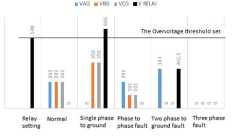
Figure 8 Voltage Function of Different Types of Disturbance
