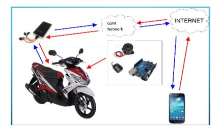
Figure 1 Architecture Design Systems Anti-Theft Vehicle Si Kemot
