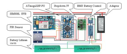
Figure 4. Hardware circuit schematic
