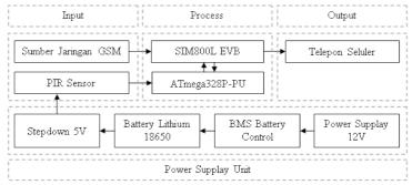
Figure 2. Block diagram instrumen device
