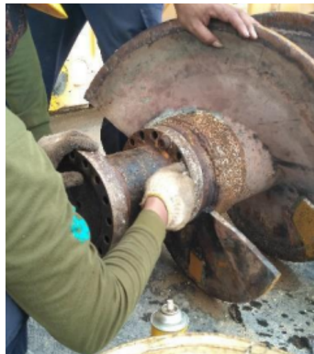
Figure 4. Inspection of intermediate shaft and screw conveyor [12]
