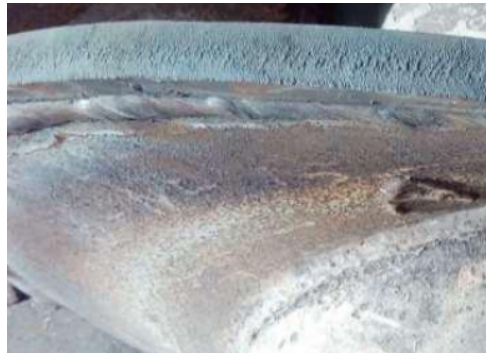
Figure 5. Examples of worn screw conveyor blades [12]
