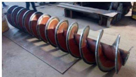
Figure 11. Screw conveyor after repaired [12]
