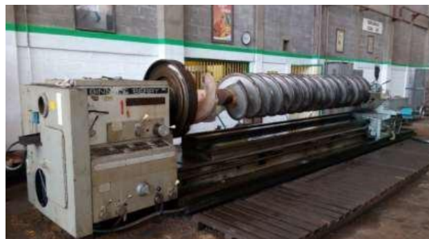
Figure 8. Reducing the diameter of the flight screw conveyor to \phi 585 mm with a lathe [12]
