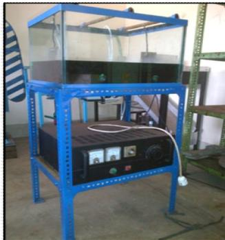
Gambar 5.1 Alat Elektroplating
