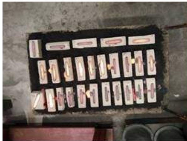
Figure 5 Casting process of samples in a mold (Tellurium powder is inserted into the mold before being cast)
