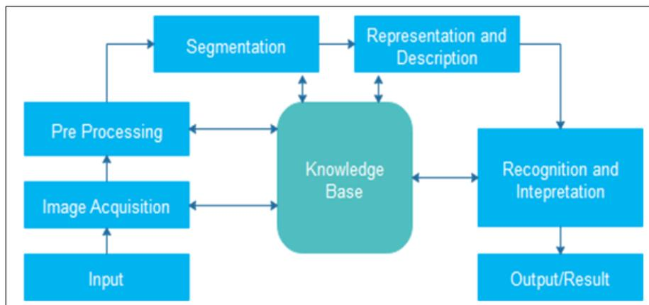
**Figure 1.** The steps in digital image processing.
