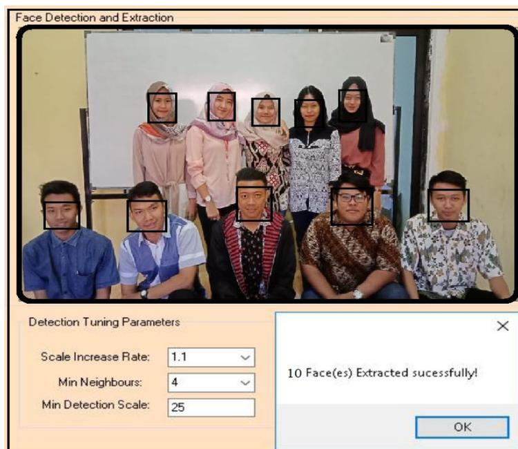
**Figure 10.** The face detection and extraction.
