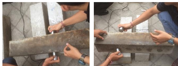
Figure 5. UPV test with direct method
