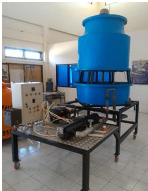
Figure 1. Induced Draft Counterflow Cooling Tower.
