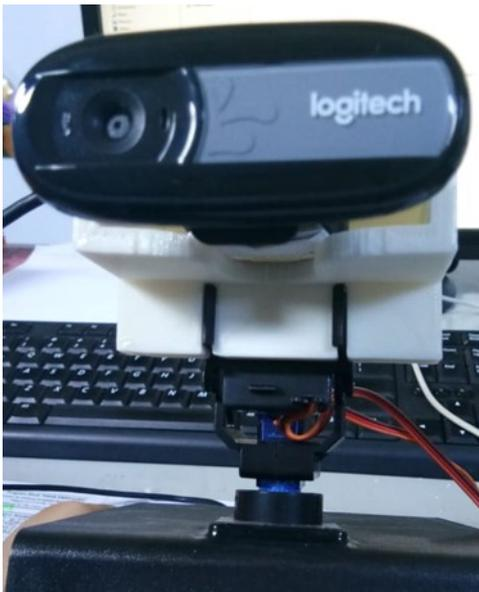
Gambar 1. *Pan-tilt camera* dan *servo bracket*
