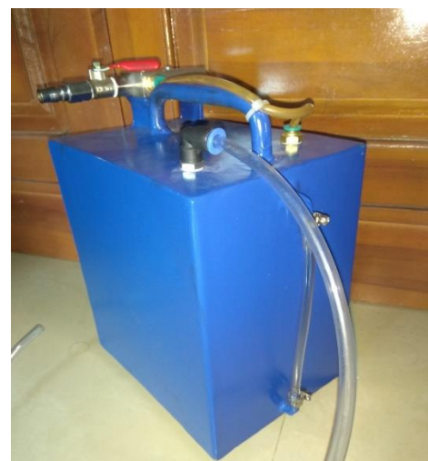
Figure 4. Production Results of the brake bleeding tool for 4 wheeled vehicles using the pneumatic system
