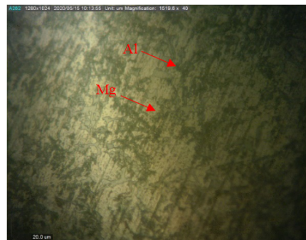
Figure 5. The Microstructure of Used Piston Castings (1500x)
