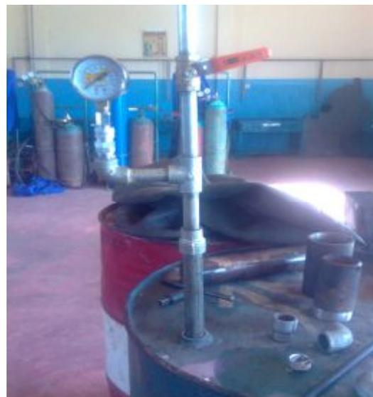
Gambar 4. Digester biogas
