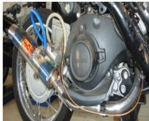
Gambar 4. Instalasi Resirkulator Gas Buang
