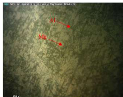
Figure 5. The Microstructure of Used Piston Castings (1500x)
