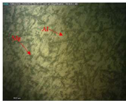
Figure 9. The Microstructure of Used Drum Castings with 0.5% Mg (1500x)
