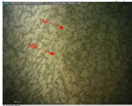
Figure 6. The Microstructure of Used Brake Lining Castings with 0% Mg (1500x)
