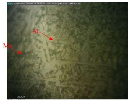
Figure 8. The Microstructure of Used Brake Lining Castings with 0.5% Mg (1500x)
