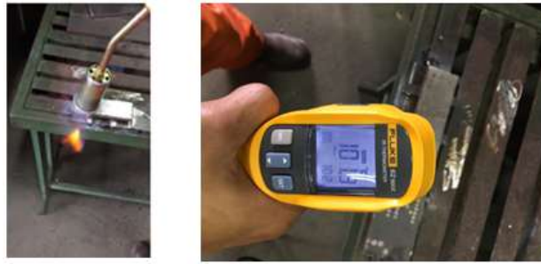
Figure 3. Preheat and SMAW Welding
