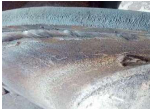
Figure 5. Examples of worn screw conveyor blades [12]
