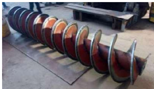
Figure 11. Screw conveyor after repaired [12]
