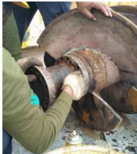
Figure 4. Inspection of intermediate shaft and screw conveyor [12]
