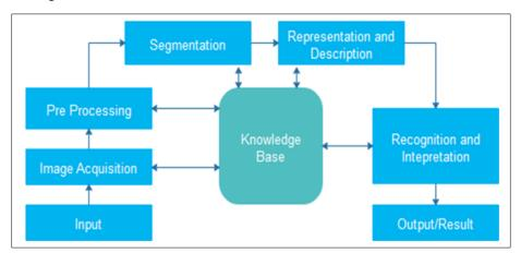
Figure 1. The steps in digital image processing.
