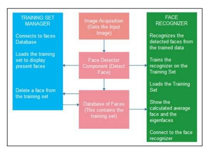
**Figure 3**. The function of the components.
