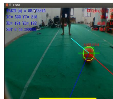
Figure 8. Ball prediction when the ball is rolling to the right.
