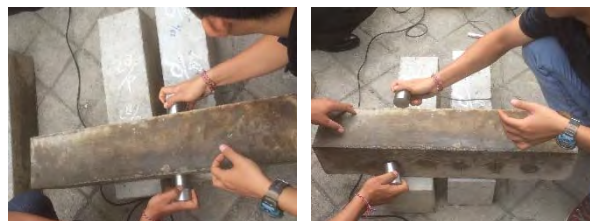
Figure 5. UPV test with direct method
