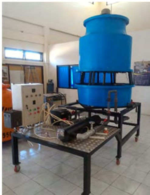
Figure 1. Induced Draft Counterflow Cooling Tower.
