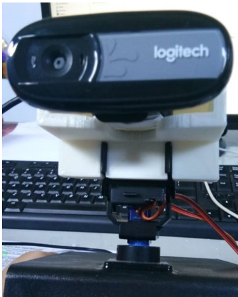
Gambar 1. Pan-tilt camera dan servo bracket
