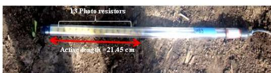
**Gambar 2.** *Photo Electronic Erosion Pin* (PEEP).
